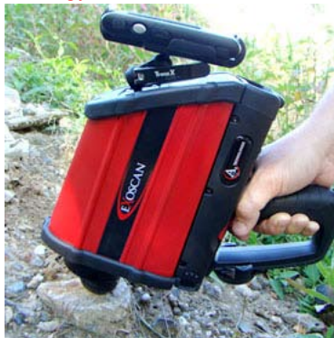
Above: In a laboratory setting, geology samples may be crushed and mixed with a non absorbing matrix, such as potassium bromide to eliminate the negative bands. In order to accomplish field measurements, the sample must be measured without preparation; therefore, the reflectance spectra is measured directly. Library matching can be accomplished with the same accuracy as laboratory data.
