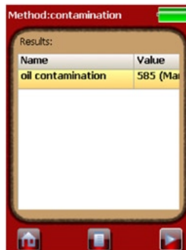
Figure 3 – Exoscan results screen showing a marginal oil contamination on a metal surface.
